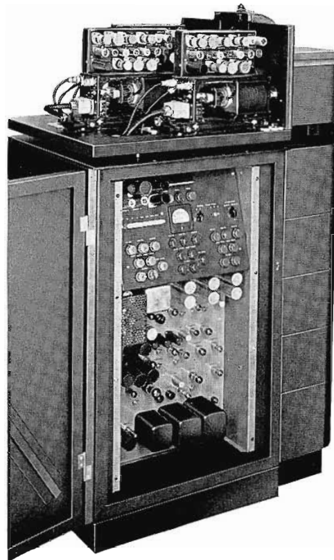
FIG. 10. Pedestal assembly supports optical system and houses camera auxiliary chassis.
