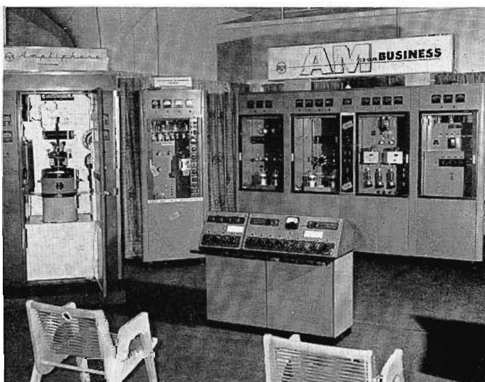
AM IS OUR BUSINESS . . . A complete line of RCA AM transmitters were shown in this area. From left to right: The power amplifier cubicle from RCA's new 50 KW "Ampliphase" transmitter; a complete 1 KW high fidelity AM Transmitter, BTA-1M; and RCA's newest 5 KW AM Transmitter, BTA-5H.
