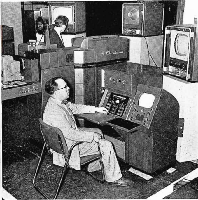
COLOR FILM SYSTEM FOR CUSTOMER INSPECTION . . . Broadcasters were encouraged to inspect and operate this TK-26 Color Film equipment for themselves. Many of them brought in their own color slides and films to run "on-camera". Note the masking amplifier located above the processing amplifier at the control position.
